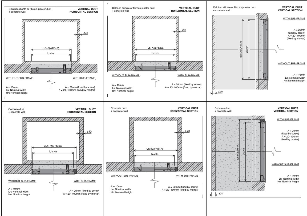
**7.5. INSTALLATION OF DAMPERS IN A DUCT HAVING SIZES ADAPTED TO THE DIMENSIONS OF THE DAMPER**
